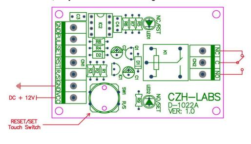
Single External Momentary Switch Control Mode: Click the external switch, relay state SET / RESET change. In the mode, on board red switch still usable.
