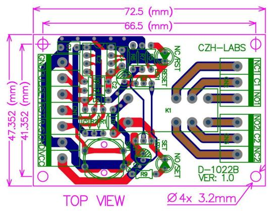
Terminal block VCC connect power supply.
